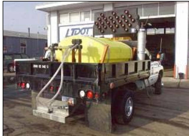
Utah DOT Maintenance Vehicle with Fog Dispersal Equipment
